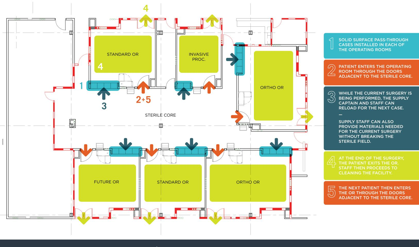
FLOOR PLAN + PATIENT FLOW WITH THE ADDITION OF SHIELD PASS-THROUGH CASES
